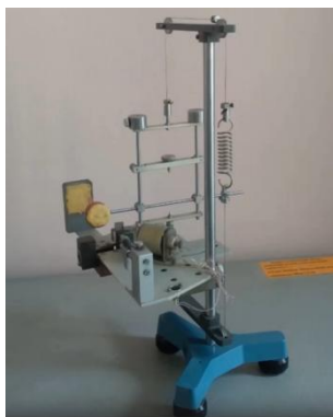
Figure 2. The equipment Atwood machine with pendulum
