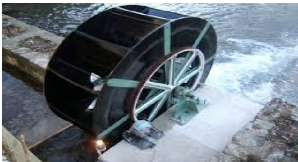
Picture-1. Micro hydroelectric power station.
