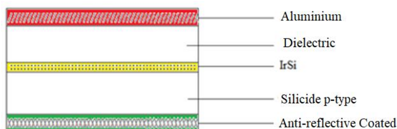
Figure 1. Structure of the photosensitive Schottky diode layer in the form of an "optical cavity"
