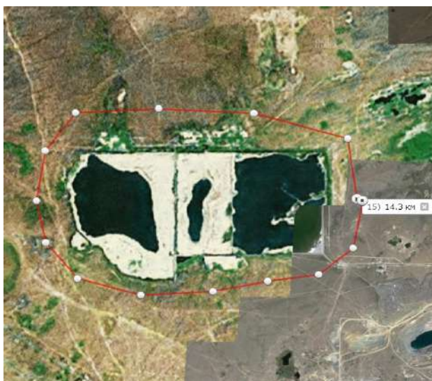
Figure 1 - Tailings storage facility for radioactive waste (red circle - border of the sanitary protection zone)
